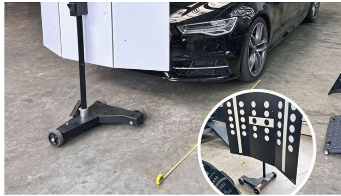
Figure 6: Incorrect setup for calibrating the front camera [30]
