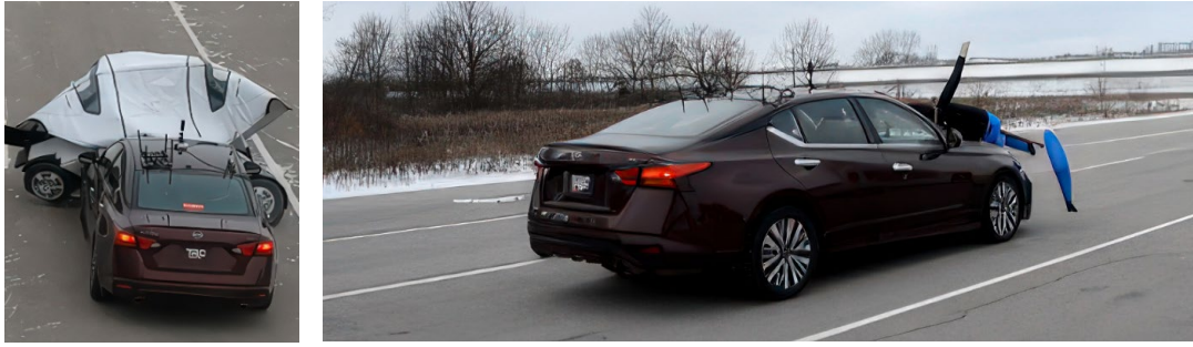
Figure 4: Vehicle collides with a vehicle target without braking (sensors misaligned, calibration missing), left; vehicle collides with a pedestrian dummy (actual condition after 12,900 miles, collision avoided following calibration), right [18]
